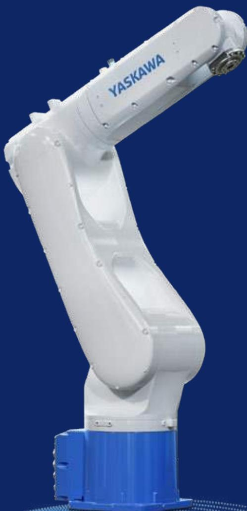
With a payload of 7 kg and a reach of 927 mm, the compact NEX7 manipulator is the right choice for a wide range of adaptive handling and assembly tasks. As part of the MOTOMAN NEXT platform, it is suitable for automation in which robots use sensors (e.g., cameras, force sensors) to detect, understand, evaluate, and autonomously respond to new situations and workpiece variants.
