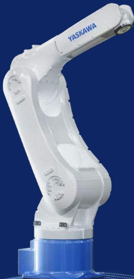
With a payload of 20 kg and a reach of 1,550 mm, the NEX20 manipulator is the right fit for a wide range of adaptive handling and assembly tasks. As part of the MOTOMAN NEXT platform, it is suitable for automation in which robots use sensors (e.g., cameras, force sensors) to detect, understand, evaluate, and autonomously respond to new situations and workpiece variants.
