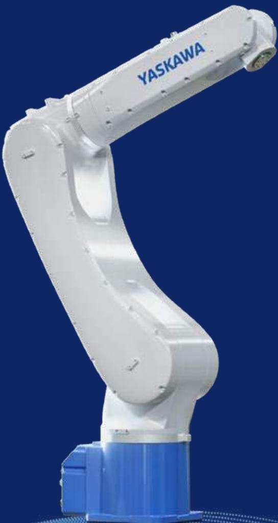
With a payload of 10 kg and a reach of 1,101 mm, the compact NEX10 manipulator is the right fit for a wide range of adaptive handling and assembly tasks. As part of the MOTOMAN NEXT platform, it is suitable for automation in which robots use sensors (e.g., cameras, force sensors) to detect, understand, evaluate, and autonomously respond to new situations and workpiece variants.
