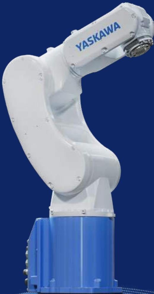
With a payload of 4 kg and a reach of 550 mm, the compact NEX4 manipulator is the right choice for a wide range of adaptive handling and assembly tasks in confined workspaces. As part of the MOTOMAN NEXT platform, it is suitable for automation in which robots use sensors (e.g., cameras, force sensors) to detect, understand, evaluate, and autonomously respond to new situations and workpiece variants.
