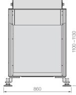
This operating platform enables the mounting of HC10-series robots in ergonomic height and provides space for the robot cable and the control MOTOMAN YRC1000. Due to the weight of 114 kg, the platform can be relocated easily with a hand pallet truck.
