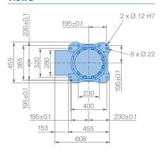
Mounting options: Floor, ceiling, wall, tilt\* Protection class: Main axes (S, L, U) IP54, wrist IP67
