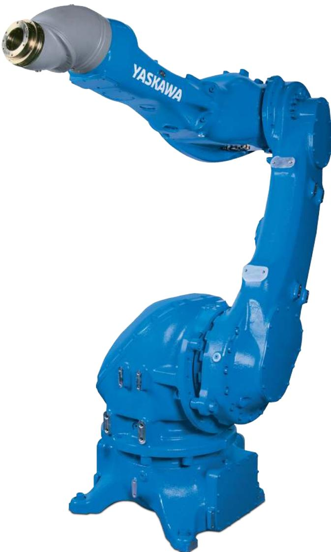
The MOTOMAN MPX2600 painting robot provides a payload of 15 kg, which enables mounting of multiple guns and large bells on this medium-sized robot. The smooth arm design with a large hollow diameter is optimal for tubing and can prevent interferences among paint and air tubes. On the U-Arm additionally paint equipment can be mounted.
