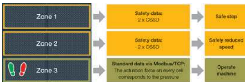
Pressure-sensitive safety mat PSENmat with integrated switch functionality.
