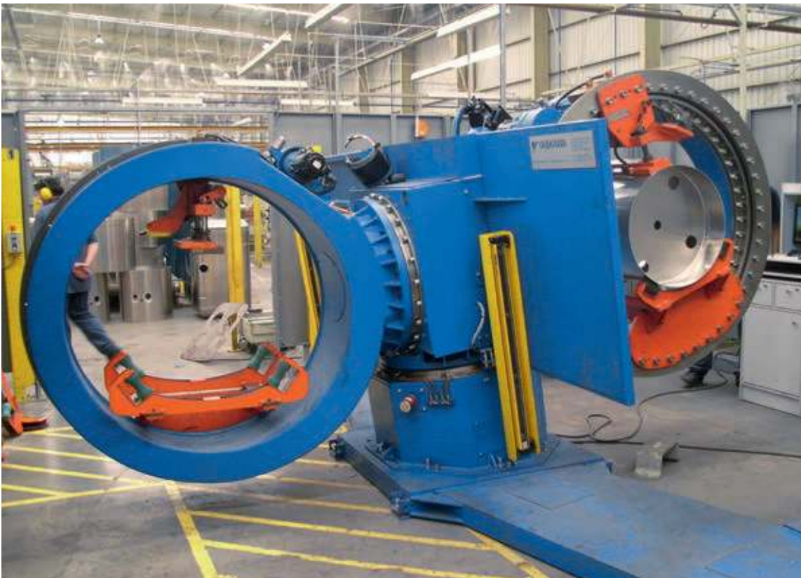
Special design: 5-axis positioning table with steady rest system for machining the end faces of long work pieces, in this case fuel tanks for trucks: welding of cover/bottom with tank casing
