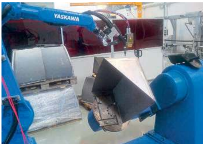
Seamtracking with MIG/MAG torch
