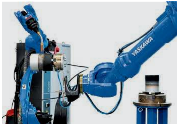
Flexible Multi-Robot system for demonstration, testing and training purposes at the Application Center in Allershausen MH225, 2x MA2010 and turn-tilt positioning table Sensor technology: tactile sensor and arc sensor
