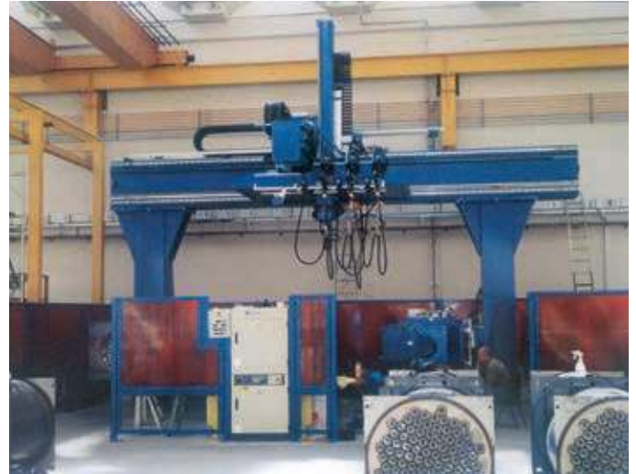
Three-axis gantry system for welding industrial heat exchangers
