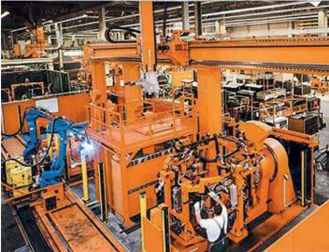
Special solution for automated MSG welding of 50 tractor cabs per day
