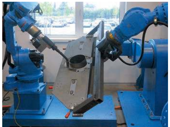
MAG welding on various housing components and subassemblies ES165 with MA1800 Sensor technology: tactile sensor and through-the-arc sensor
