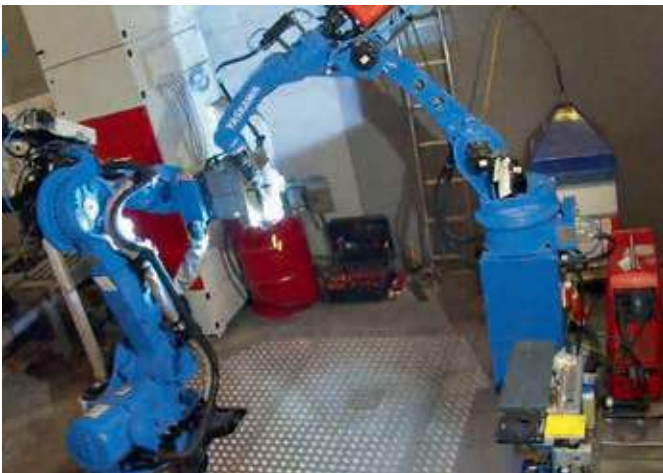
MAG welding on bulk material containers MH400 with MH50-30 Sensor technology: vision system, MOTOSense SeamFinder and tactile sensor
