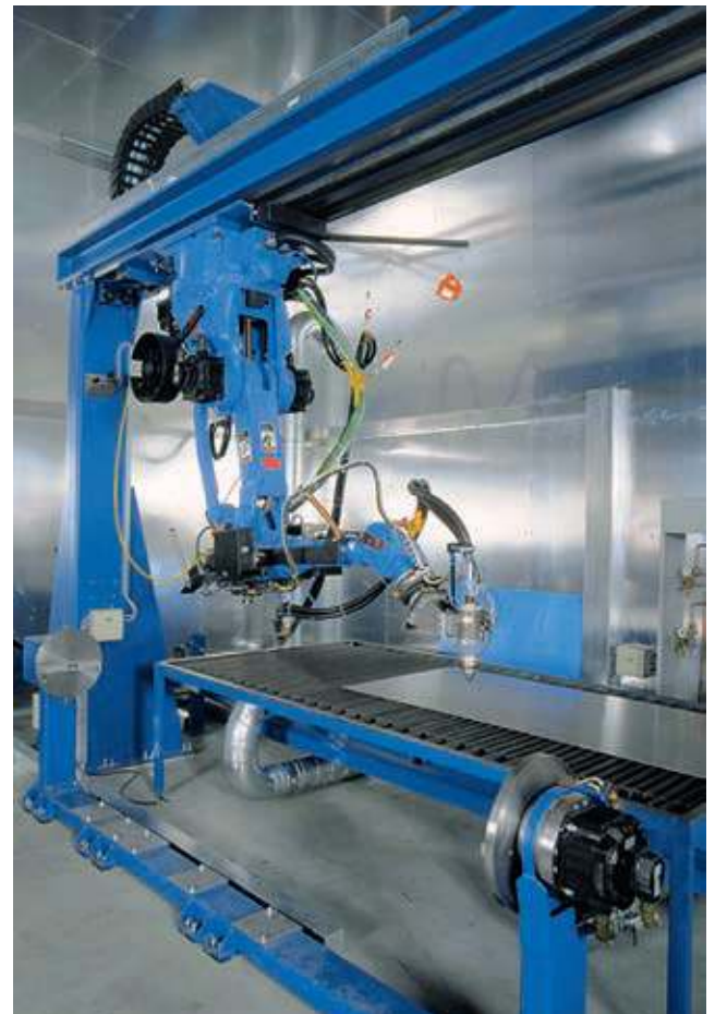
Laser cutting cell: 50 kg robot on gantry track
